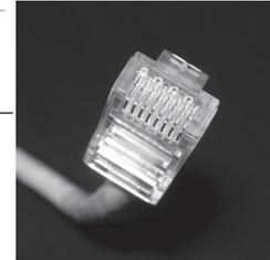
The type of cable is known as twisted pair. It has an RJ-45 plug on the end, which is molded so it can only connect one way to the RJ-45 port. It also has a tab that locks it in place. The RJ-45 plug is slightly larger than a telephone cable's RJ-11 plug, but looks very similar. Another difference is that the phone plug usually has four wires, whereas the RJ-45 plug has eight.
