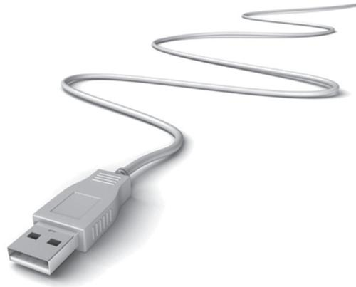
USB version 1.0 had data transfer rates of 1.5 megabits per second (Mbps) at low speed and 12 Mbps at full speed.
