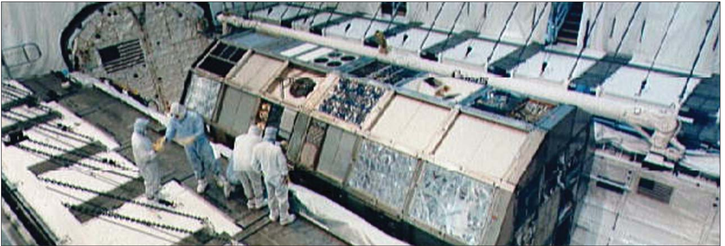
Noticeably weathered, the Long Duration Exposure Facility (LDEF) remained remarkably intact after six long years in space. NASA photo.
